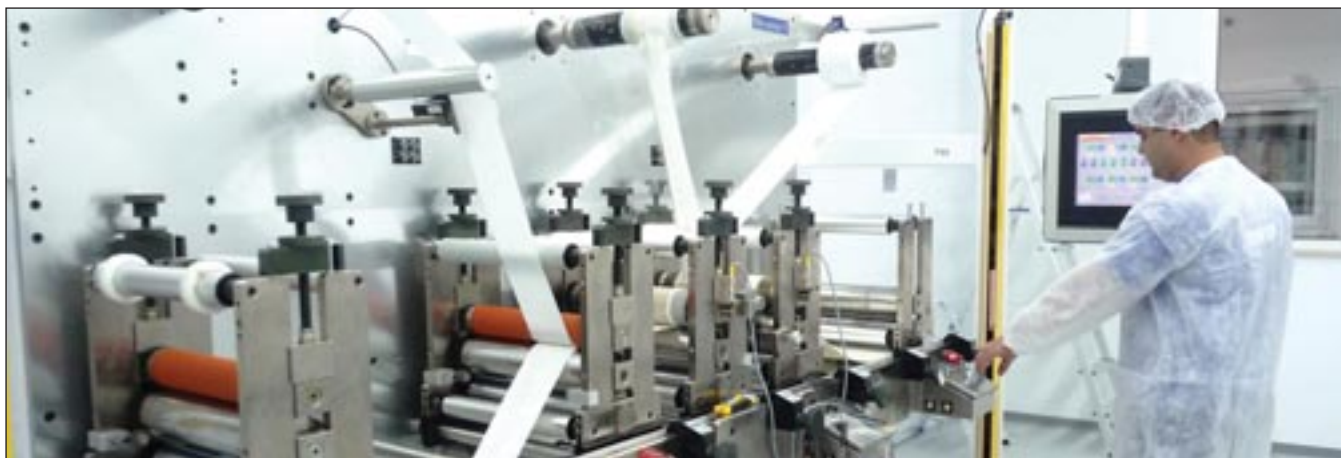
These rotary converting machines in Pronat Medical's cleanroom are used for mass production of wearable devices. (Credit: Pronat Medical)
