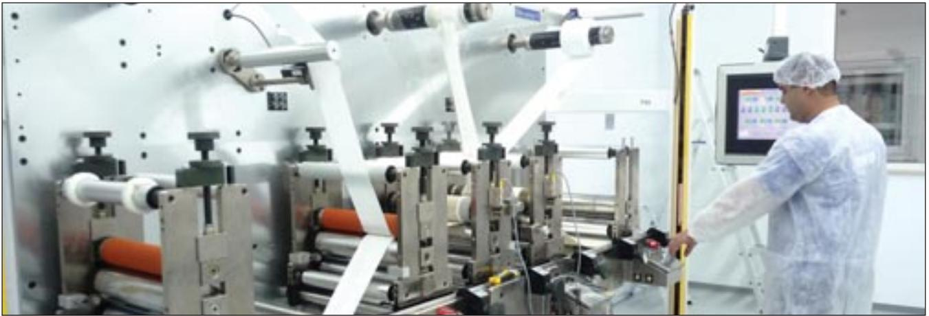
These rotary converting machines in Pronat Medical's cleanroom are used for mass production of wearable devices. (Credit: Pronat Medical)
